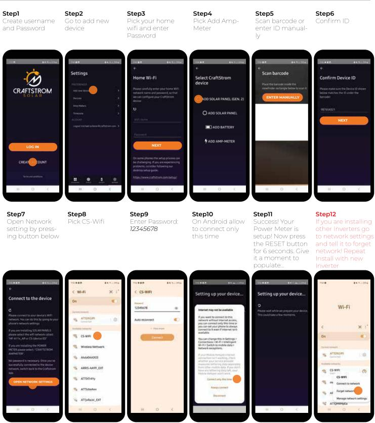
After the installation process was successful please push the rest button for **1** second. the Data should now display on dashboard!
