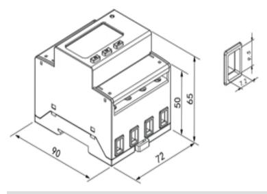
The CraftStrom PowerMeter is a power measuring device that is installed either on standard DIN rails in distribution boxes; or, if there is no space or no DIN rail available, there is also the option to purchase the PowerMeter with induction sensors (CT brackets}.
