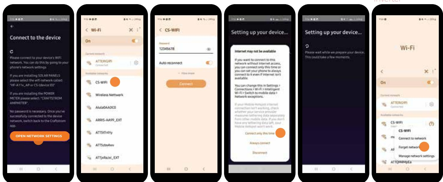
If the Inverter does not show up on the panles page, then go back to Settings - Devices delete the ID number and repeat the installation - remember to forget network (CS WIFI) in network settings before you reinstall! To reset wifi module on Inverter - press silver button next to antennas for 1 second...
