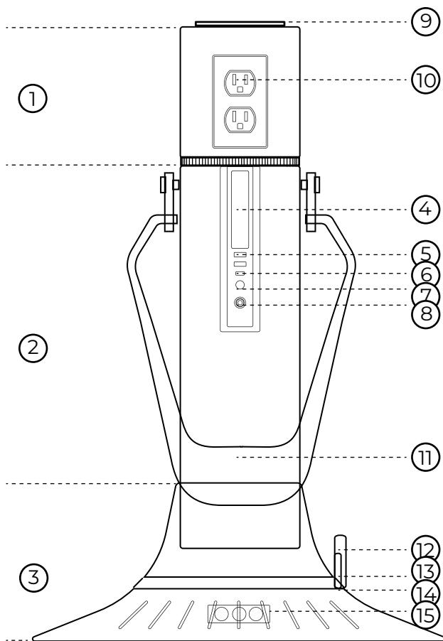
1. Detachable Off-Grid Inverter & Quick Release Ring
