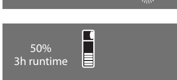
Battery in OFF - GRID mode & idle. 50% charged with a runtime of 3h.
